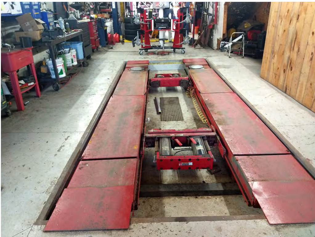
Vehicle alignment service bay.
